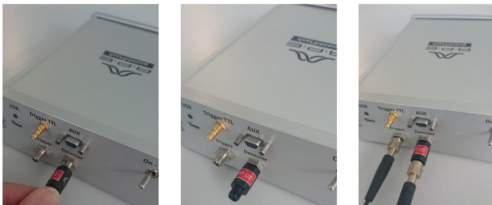
Figure 3 (left to right): screw attenuator directly on detector output, mount fiber on attenuator
